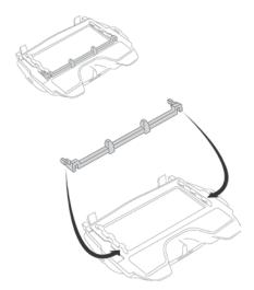
The distance bar only needs to be attatched to the 3M<sup>™</sup> Speedglas<sup>™</sup> Welding Filters 9100X and 9100XX to prevent the inner protection plate from being scratched against the rail.
